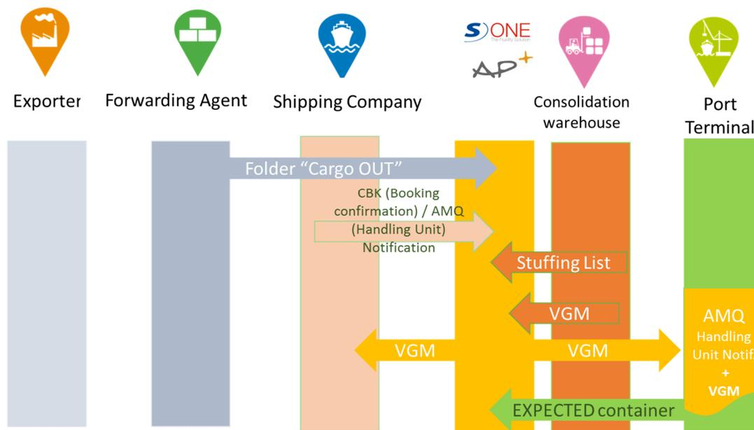
Bulk containers are also concerned by the VGM procedure. The weight of the LDE is not sufficient. It is essential to include the weight of the dunnage (material) and the tare mass of the loaded container as part of the VGM value.
